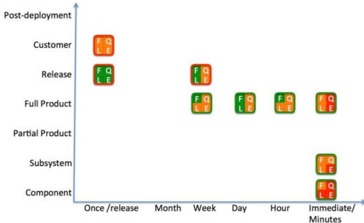
Figure: An example CIVIT model. The colors in the boxes indicate the test coverage for functional requirements (F), quality requirements (Q), legacy functionality (L) and edge cases (E), ranging from no testing (red), less than 30 percent (orange) to full coverage (green). The colors of the borders around the boxes indicate the level of test automation, from none (red), less than 30 percent (orange) to full (green).
